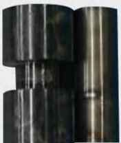
Identical part treated using competitive quench oil – showing oxidation and excessive discoloration.
